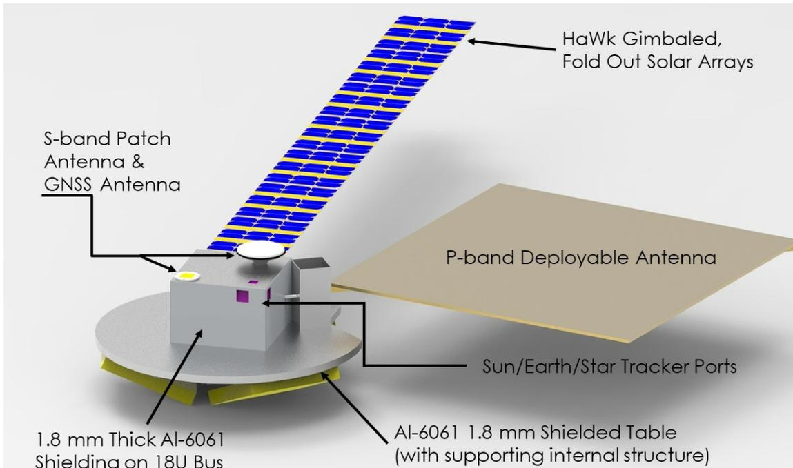
Figure 15: Isometric View of Deployed Spacecraft
