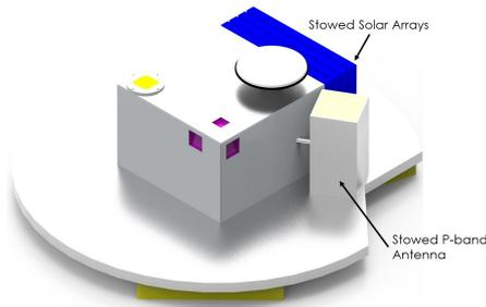
Figure 13: Isometric View of Stowed Spacecraft
