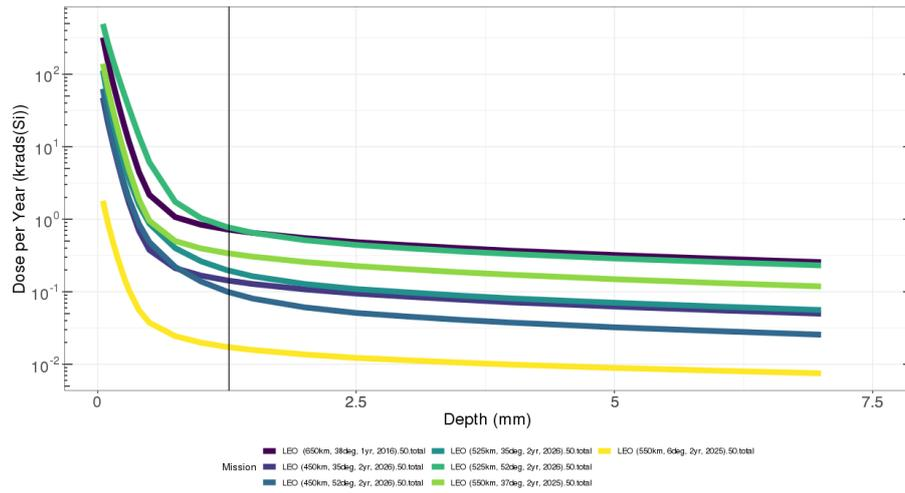
Figure 34: Radiation Dose per Year of Satellites in Similar Orbits as the 550 km Plane (Highlights the Recommended Minimum Radiation Shielding Depth)
