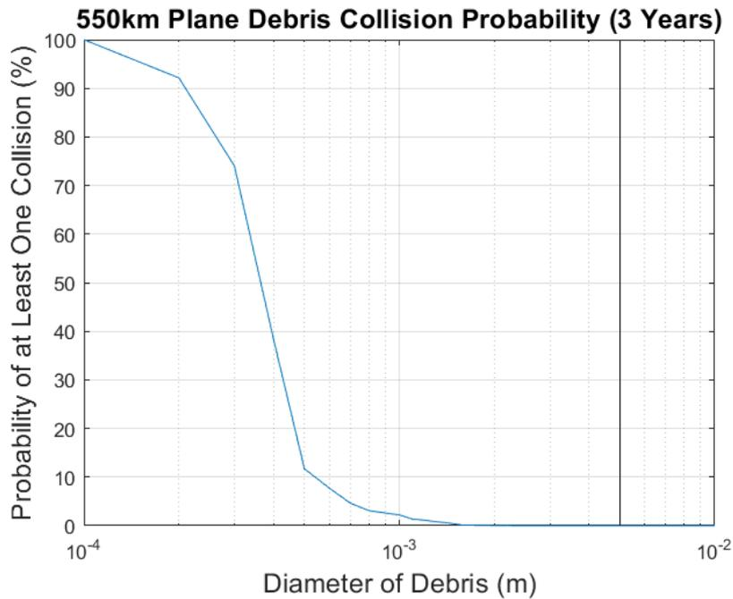
Figure 32: Probability of Collision with Debris at the 550 km Orbit (Highlights Debris with a Diameter of 5mm)
