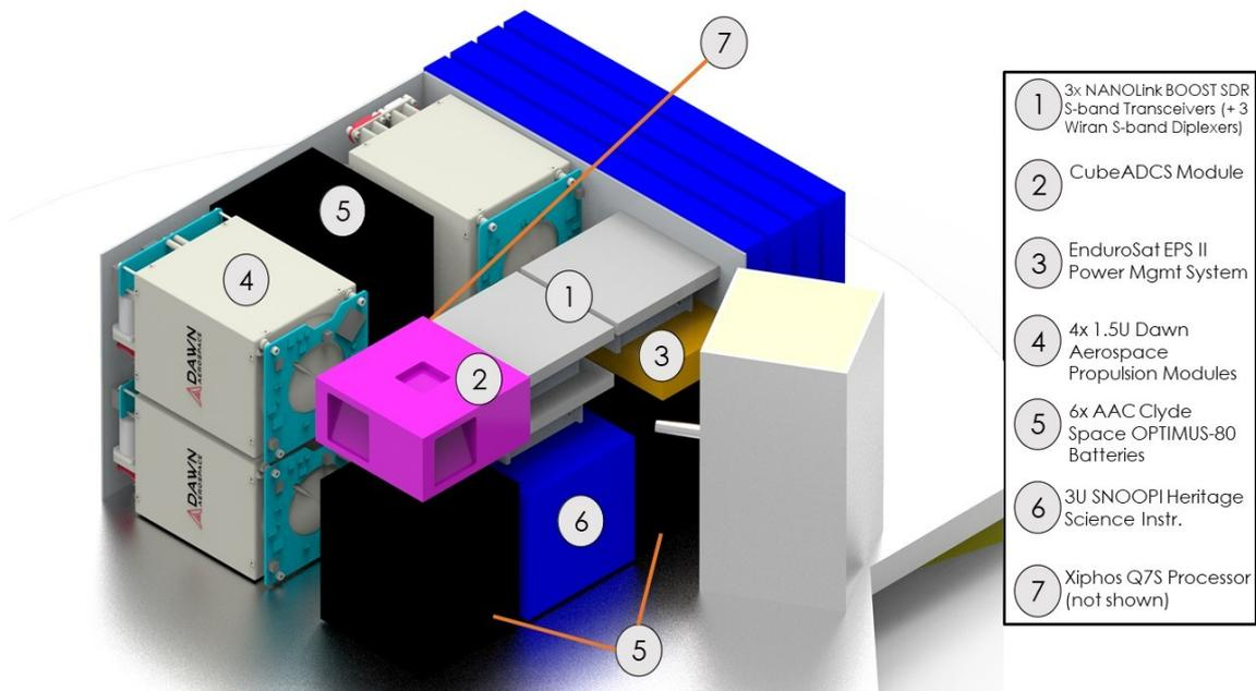
Figure 18: Internal Instrument Configuration
