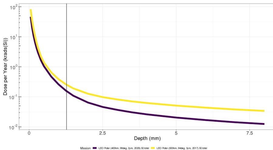
Figure 33: Radiation Dose per Year of Satellites in Similar Orbits as the 350 km Plane. Highlights the Recommended Minimum Radiation Shielding Depth
