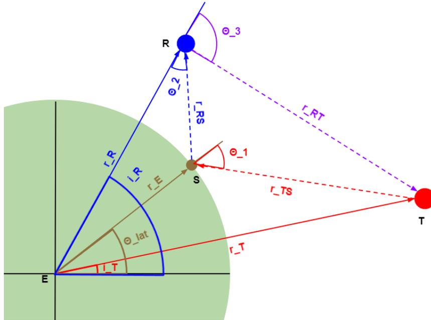
Figure 2: Representation of the Geometry of the MoIST Receiver (R) Detecting the Specular Point (S) whilst Maintaining a Direct Signal with the Transmitter (T).
