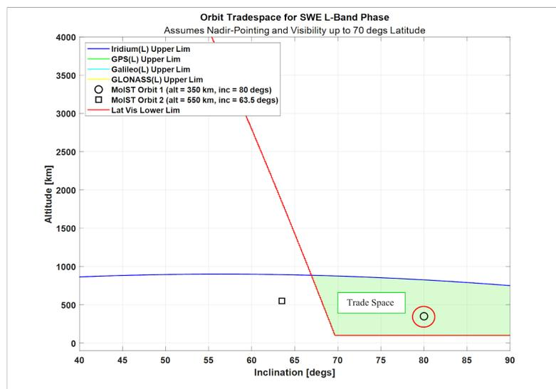
Figure 4: Region for Which High Latitudes of the Earth can be Observed Using L-Band Constellations
