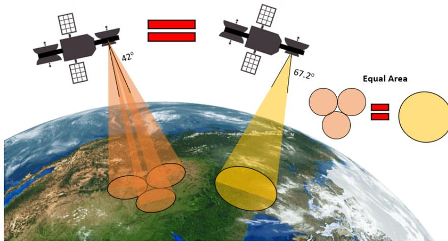
Figure 8: How Adding More Antennas can Help Improve the Revisit of the Freeze-Thaw Science Measurement (red). How These Additional L-band Antennas are Modeled in the Code (yellow)
