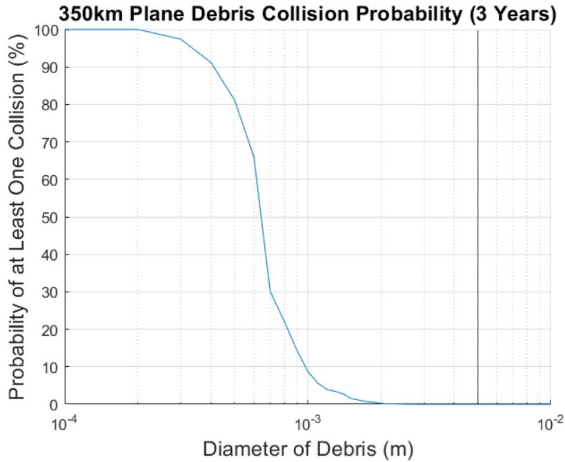
Figure 31: Probability of collision with debris at the 350 km orbit. Highlights debris with a diameter of 5mm
