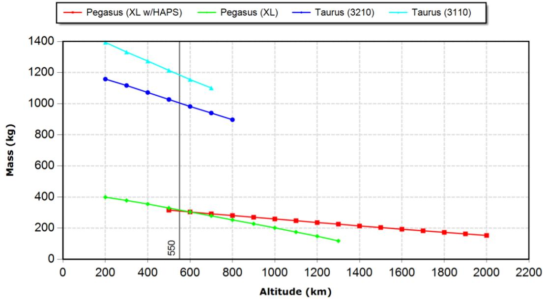
Figure 10: NASA Vehicle Performance Analysis (550 km Orbit Plane)
