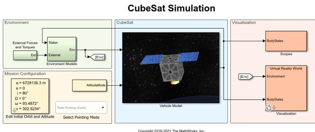
Figure 22: Simulink Model Used to Determine the Requirements for the ADCS System
