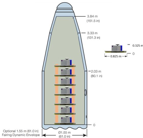
Figure 11: Minotaur Payload Configuration
