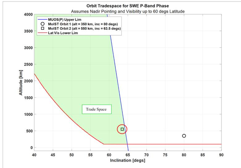
Figure 3: Region for Which High Latitudes of the Earth can be Observed Using MUOS
