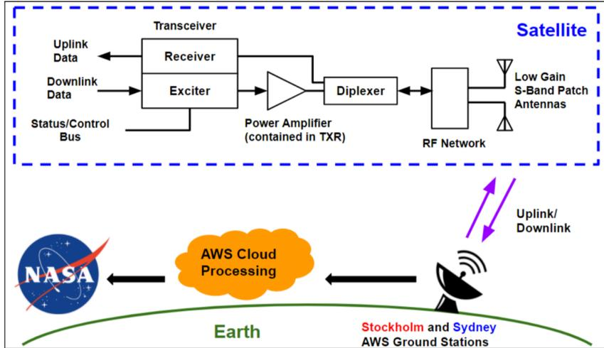
Figure 19: Data Transmission Architecture Flowchart
