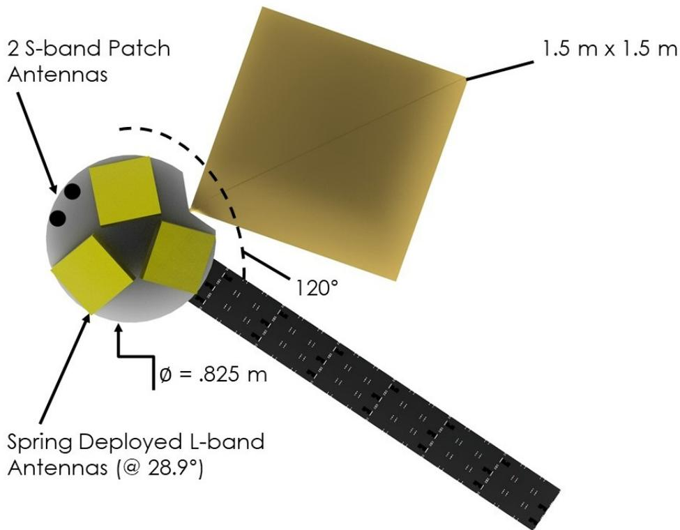
Figure 17: Bottom Profile of Deployed Spacecraft
