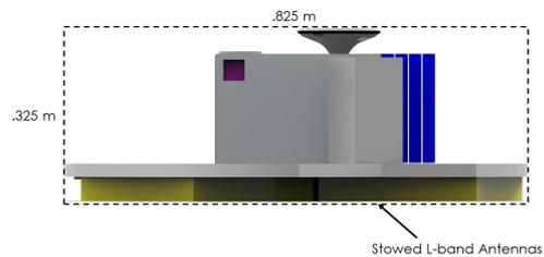
Figure 14: Profile View of Stowed Spacecraft
