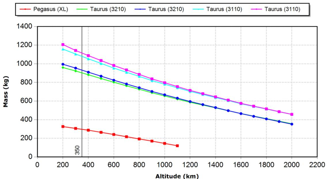
Figure 9: NASA Vehicle Performance Analysis (350 km Orbit Plane)
