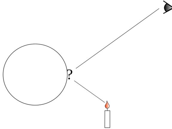
Figure 7: Visualization of a Reflection off a Sphere Used in the Alhazen-Ptolemy Problem
