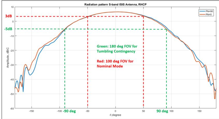
Figure 20: S-Band Patch Antenna H- and E-Plane Gain Patterns
