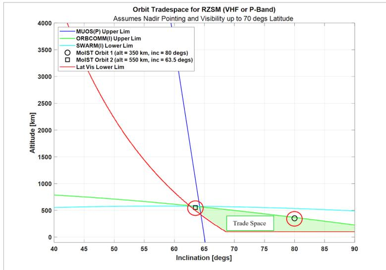
Figure 5: Region for Which High Latitudes of the Earth can be Observed Using P and VHF/I-Band Constellations
